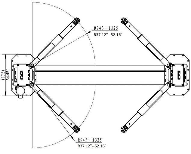
Fig. 3 (Column / Floor Layout)
