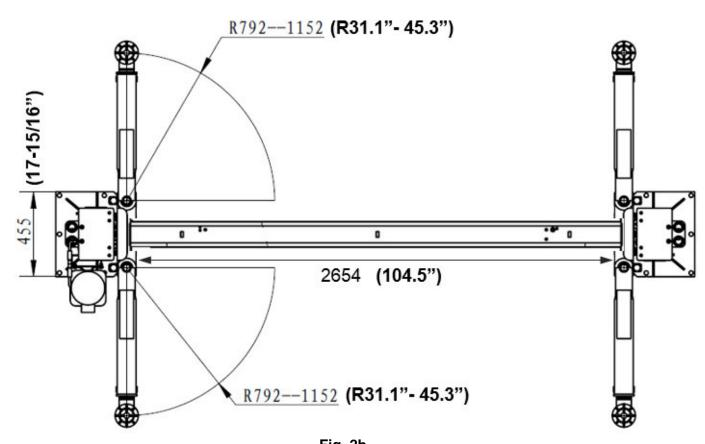
Fig. 2b (TP9KSCX - Symmetric Lift)
