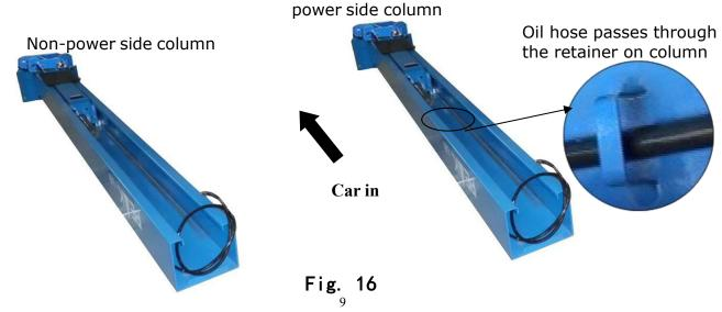
E. Install the cylinder and connect the oil hose to the cylinder.
