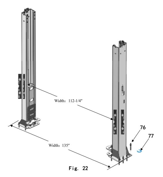
\*Note: The anchor bolt is knocked into the ground at least 3-1/2".
