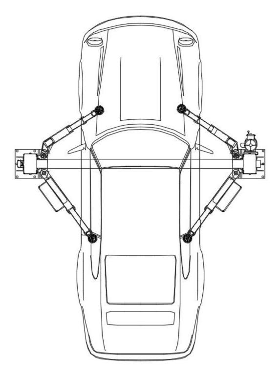
Swing and extending the arms to the lifting point of vehicle
