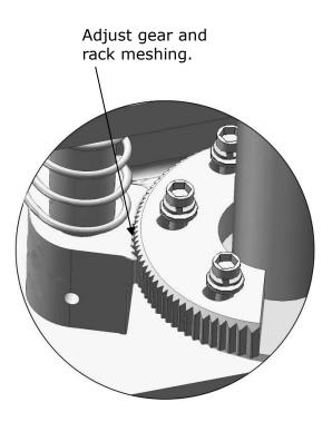
Lock the screws by wrench after the gear and rack are in good meshing condition
