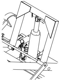
Figure 4: Inserting Bottle Jack Pin.
