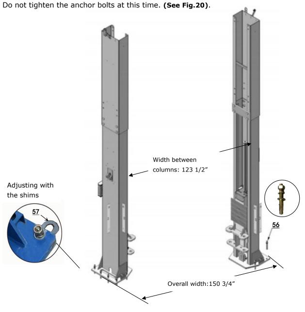
**Note:** Minimum embedment of Anchors is 5 7/8"(150mm).
