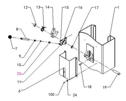
Fig. 24 Power-side safety device
