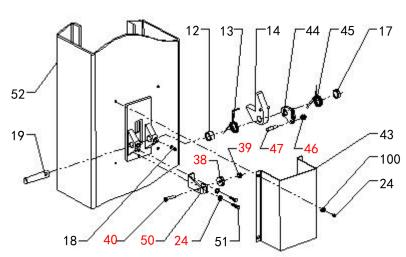
Fig. 25 Off-side safety device
