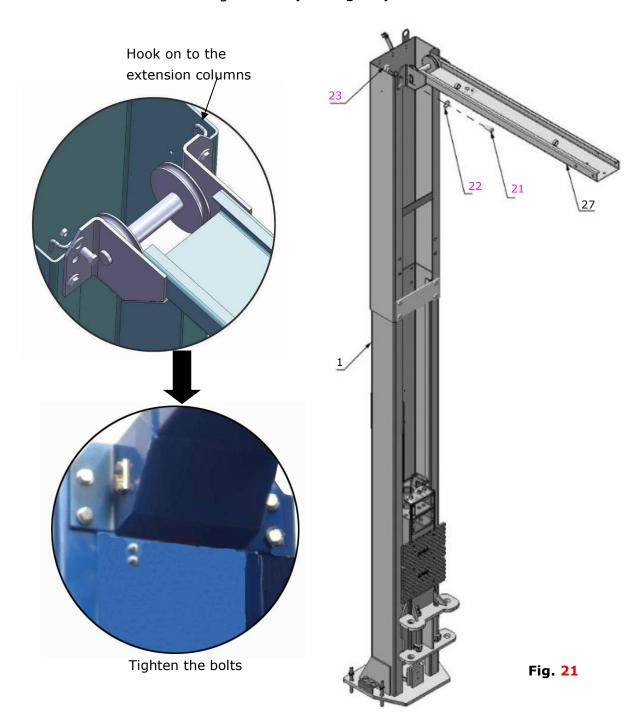
2. Assemble overhead top beam, tighten the columns anchor bolts (See Fig. 22).
