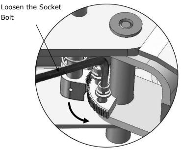
Use the 8<sup>#</sup> socket head wrench to loosen the socket bolt Fig. 35
