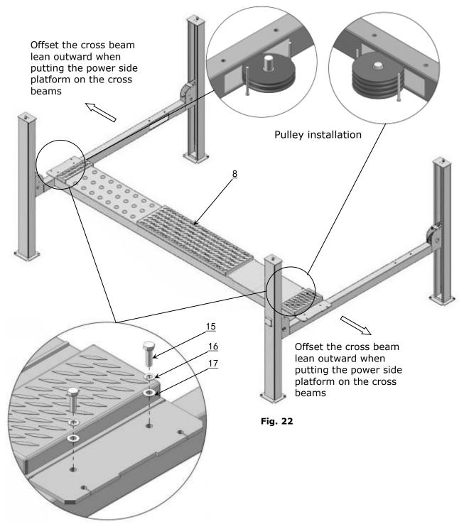
Install the power side platform and screw up the hex nuts M16\*40
