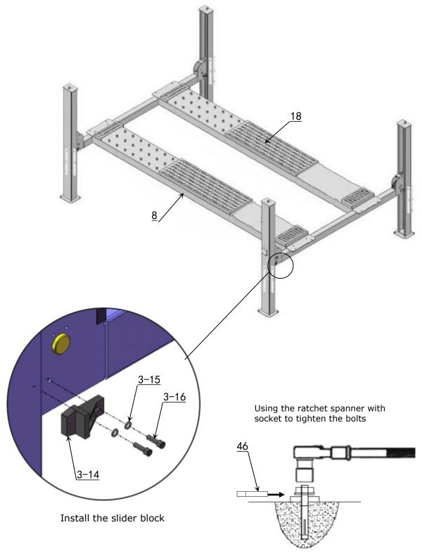
Note: The tightening torque for the anchor bolt is 150N.m
