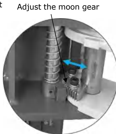
2.2 Follow the arrow direction to adjust the moon gear Fig.43
